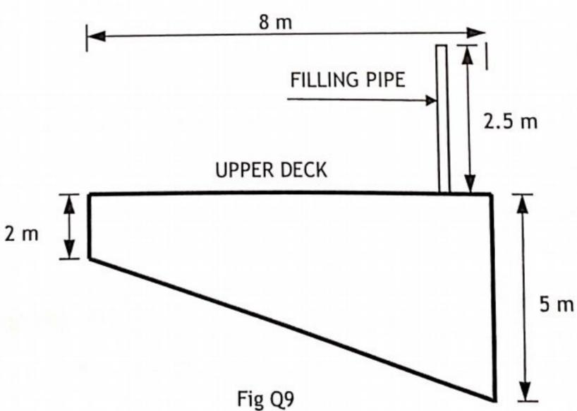
The tank is tested by filling with fresh water of density  $1000 \text{ kg/m}^3$  through a filling pipe to a head of 2.5 m above the upper deck.
