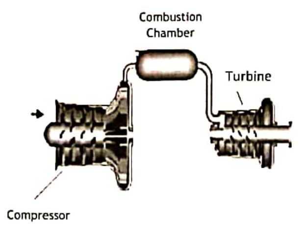
The compressor in an open gas turbine cycle receives air in at a pressure and temperature of 1.054 bar and 17°C and delivers to the combustion chamber at a pressure of 5.8 bar and 210°C.
